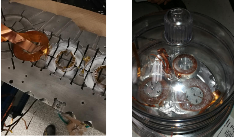
Figure 3.8: Right: Epoxy was used to fill in the gap between layers of the wound coils, which fixed their form as well. They typically took several hours to cure. So before that, we put them in a vacuum bell and extracted any bubbles that were inside the glue. Left: we tried fitting the coils into the aluminum coil holder. Before finally putting them in, we added a layer of thermal paste on the holder to fill in the gaps and allow for better heat conduction.
