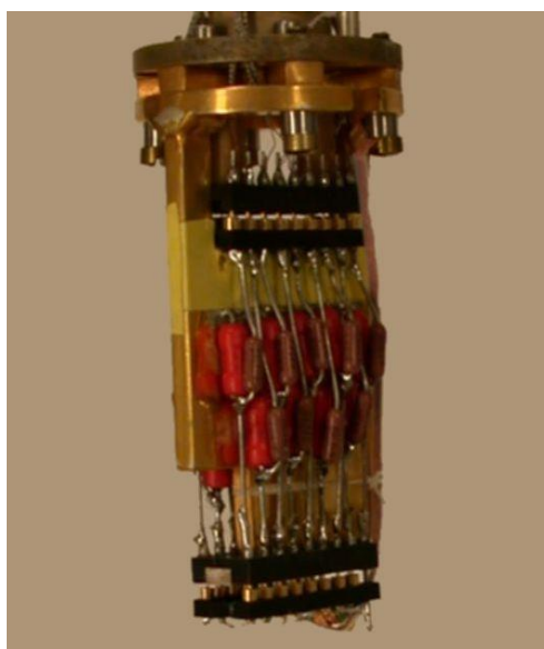
Figure C.7: Photo of the KelvinOx 25 sample mount attached to the tailpiece.
