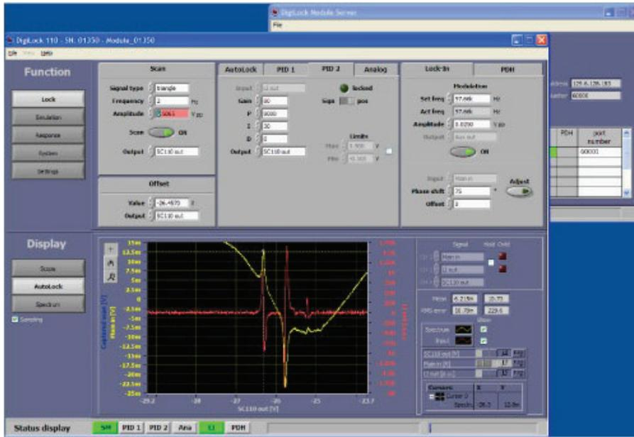
Figure 4.3: A screen shot of our absorption (yellow) and error signal (pink) for locking the potassium laser with Digilock software connected to a Toptica Photonics Feedback Controlyzer connected to our repump laser system.
